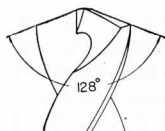
Fig. 52. Crankshaft-Point Deep-hole Drilling (Note Heavy Web)
