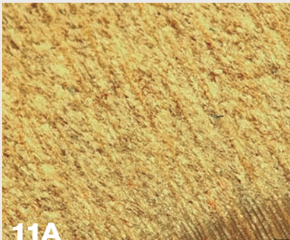
Magnification 100X, wood surfaces cut with PM 2030 gouge.
